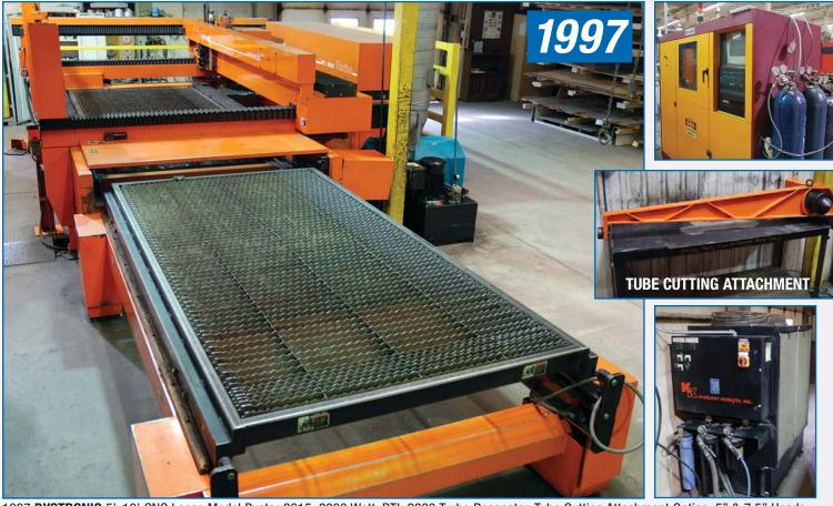
1997 BYSTRONIC 5'x10' CNC Laser, Model Bystar 3015, 2800 Watt, BTL 2800 Turbo Resonator, Tube Cutting Attachment Option, 5" & 7.5" Heads, Travels: X- 118.1", Y-59.1", Z-8.7", Table Size 128" x 66", Standard Chuck 3.9" – 13.4", Locking Length 102.4", Max Cutting Speed 1,968 IPM, Max. Positioning Speed 5,551 IPM, Material Thickness Capacities: Structural Steel .78", Stainless Steel .47", Aluminum .39", Max. Table Load 1,653 lbs, Koolant Koolers Chiller, sn K960103
