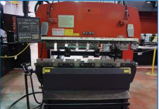
AMADA 88 TON X 6'10". CNC HYDRAULIC PRESS BRAKE, MODEL RG80S
