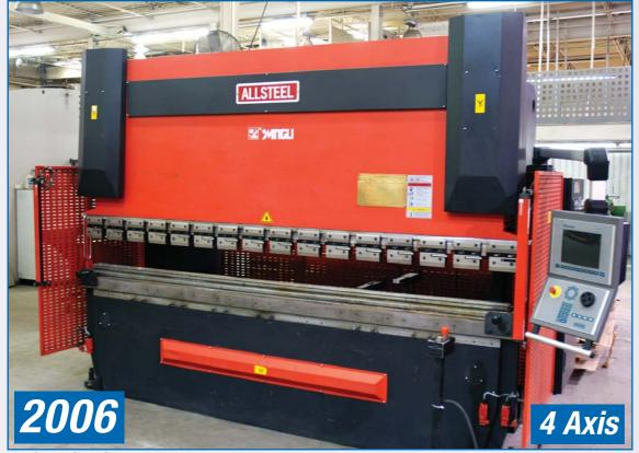
ALLSTEEL/YANGLI 110 TON X 10' CNC HYDRAULIC PRESS BRAKE, MODEL MB8-100/3200
